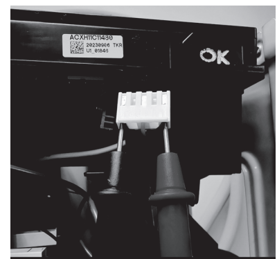
Measure the winding resistance from fan motor connector
